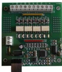
IN8 is a low size auto powered control unit equipped with USB interface. IN8 can check eight galvanic isolated inputs: on each input it is possible to apply voltages regardless from the USB ground, with a maximum voltage of 30V.
