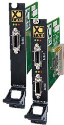
PXI boards for the Boundary Scan test and PXI rack equipped with hardware modules
