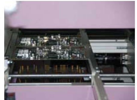
Conveyor unit with synchronous AC motors for accurate stop and automatic wide adjustment.
