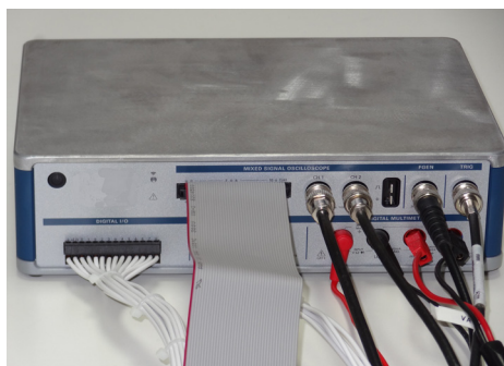
Detail of the Measurement Unit (P/N AD539) included in the 6TL-08 UNIVERSAL, with FGEN, DMM, Scope DIO and Logic Analyzer.
