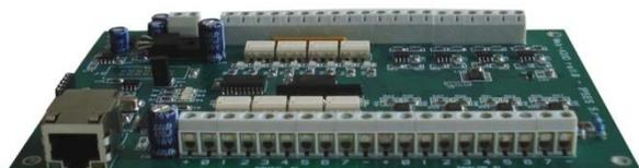
WEB-ADIO is a card to manage 8 optocoupled digital inputs, 8 analogical inputs, 8 optocoupled digital outputs and 8 analogical outputs with Ethernet interface, equipped with a web, a telnet and an SNMP servers. The WEB server allows to connect and to manage the card using any web browser (i. e. Internet Explorer and Firefox), with no needs to install a software on your PC Beside, the card can be connected directly to a switch or to a router with no need to use a PC.
