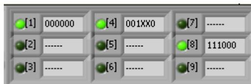
Picture 14: output programming status; green light indicates which one of the output lines is active.
