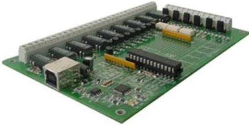
IO-69-USB is a self-powered card to manage six optocoupled inputs and nine relay outputs with USB interface.
