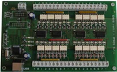
IO1616 is a self-powered card to manage sixteen optoisolated inputs and sixteen optoisolated outputs with USB interface. The model is available also with RS232 interface, in this case the card needs external power supply.
