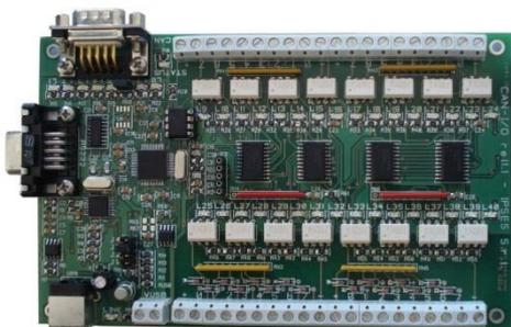
CAN-I/O is a control unit equipped with CAN, USB and RS232 interfaces to manage sixteen optocoupled inputs and outputs. The card can work as standalone device on CAN BUS. Its configuration is achieved either through USB (in this case the board is self-powered) or through RS232 interface. Easy to use and to configure, thanks to the provided software, CAN-I/O is the right answer to the need to acquire and to drive digital signals through already existing CAN bus.
