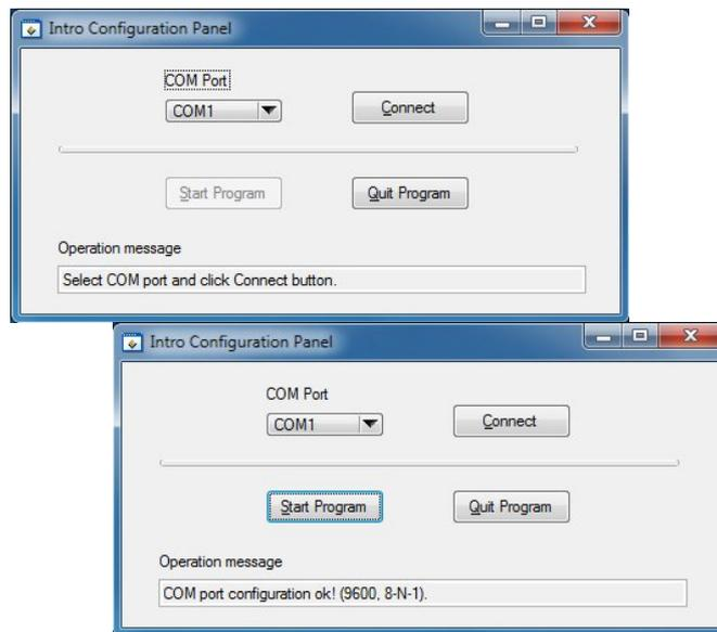
Picture 5: a) start connection window; b) COM port correctly configured.
