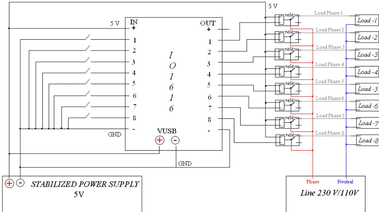
Picture 4: Stand alone mode connections (without PC).
