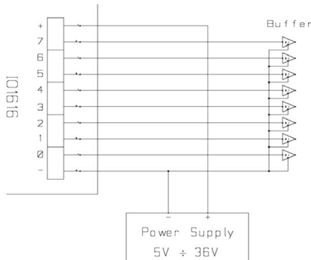
Picture 2b: diagram of the output connections.
