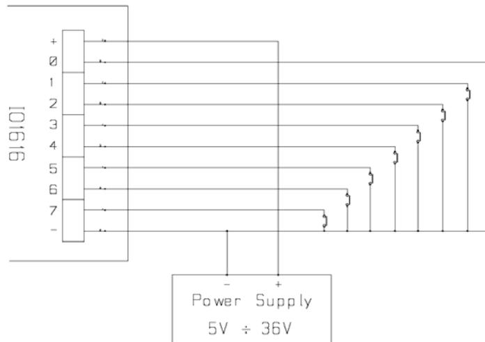
Picture 3a: diagram of input implementation.
