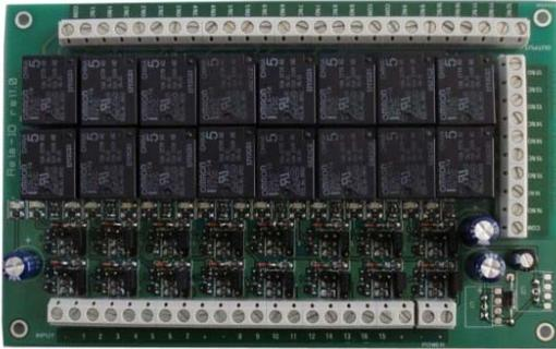
RELAY I/O(-SEL) is an expansion module with 16 digital inputs that can control 16 SPDT relay outputs 5A @ 250VAC or 5A @ 24VDC each
