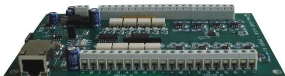
WEB-ADIO is a card to manage 8 optocoupled digital inputs, 8 analogical inputs, 8 optocoupled digital outputs and 8 analogical outputs with Ethernet interface, equipped with a web, a telnet and an SNMP servers. The WEB server allows to connect and to manage the card using any web browser (i. e. Internet Explorer and Firefox), with no needs to install a software on your PC. Beside, the card can be connected directly to a switch or to a router with no need to use a PC.
