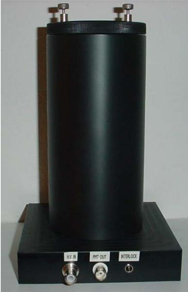
The Head-on 52 mm Photomultiplier (PMT) is a detector unit generally used in alpha particle counting systems.
