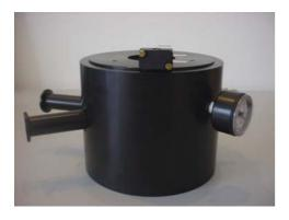
High vacuum TL oven is conceived to heat samples during thermoluminescence analyses. Warming is achieved through a heating strip in an inert atmosphere obtained thanks to a continuous air extraction by a vacuum pump and following introduction of nitrogen.
