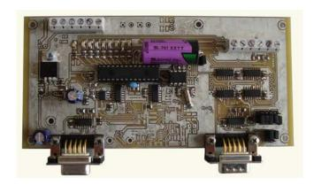
**SerialLogger** is a board which can monitor, ask and store data by a simple RS232 serial interface.
