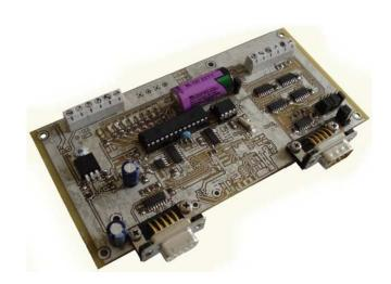
SerialLogger is provided with a Windows tool software which manages all its functions.
