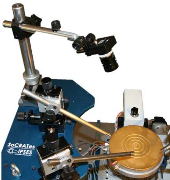
SoCRATes: thermostated wafer chuck and NIR camera
