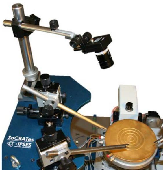
SoCRATes: portawafer termostato e telecamera NIR
