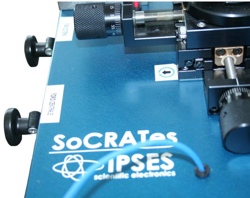
Figure 8 – Button valves for operating the vacuum system on the wafer chuck.
