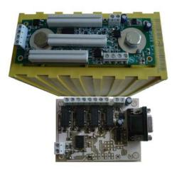
**LiBRA** is an innovative lithium battery management system allowing optimal charge and discharge, temperature control and balancing of every single cell. **LiBRA protects battery** preventing going under and over cell voltage current and temperature limit. Besides, the system allows **battery enhancement** and **complete monitoring in real time**.
