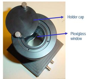
To place the sample inside the Photomultiplier (PMT), take off the sample holder (the upper part of the PMT) from the housing as shown in the picture below (Fig. 1)
