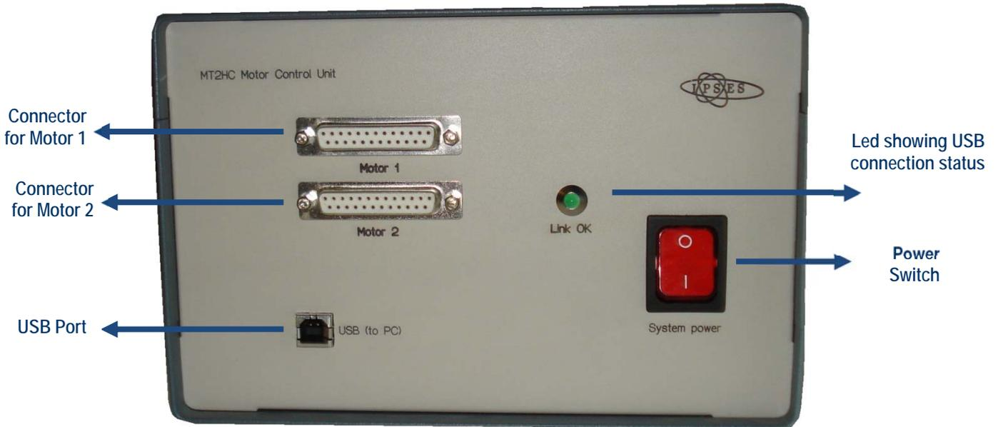
Picture 2a: MT2HC-BOX – Position of connectors and USB Port
