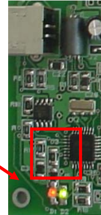
Picture 2: exchanging data and established connection LEDs.
