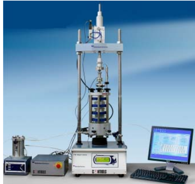
Dynatriax system by Wykeham Farrance, Soil Mechanics Division of CONTROLS.
